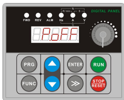
Fig 3-1 Power-on Parameter Display Initialization Display "P.OFF"
