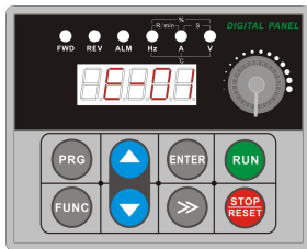
Fig 3-4 Fault Alarm Display of Over current during Accelerating
