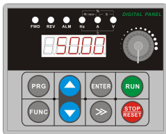
Fig 3-2 Stop Status Parameter Display Display Set Frequency "50.00"
